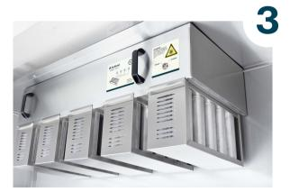
**3.** UV light and ozone are produced by the fluorescent lamp in the filter housing's reaction chamber. When the air flow comes into contact with the UV light and ozone, the remaining grease and odours are broken down
